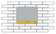
3. Screw enclosure in wall on left and right side with countersunk screws.
