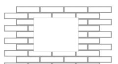
Dimensions of cutout in wall (WxHxD): 10.5 inch Domo: 305x220x50 mm Cable input on bottom in middle!
