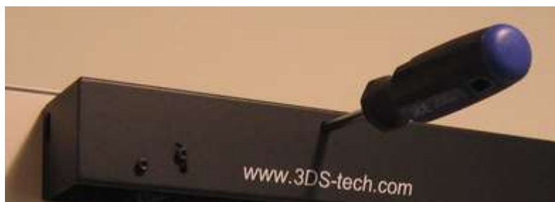
Figure 4: Tightening the Camera Bar Mounting Screws
