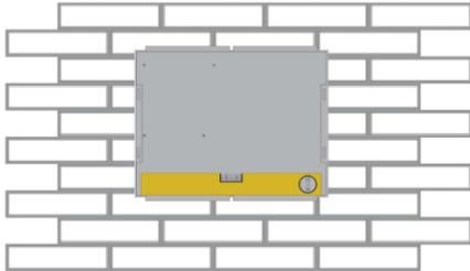
3. Screw enclosure in wall on left and right side with countersunk screws.
